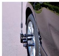
Easy to mount on car's wheel (adjustable to every car model), connect this odometer to the Ekinox-N/D to increase car's trajectory accuracy.
